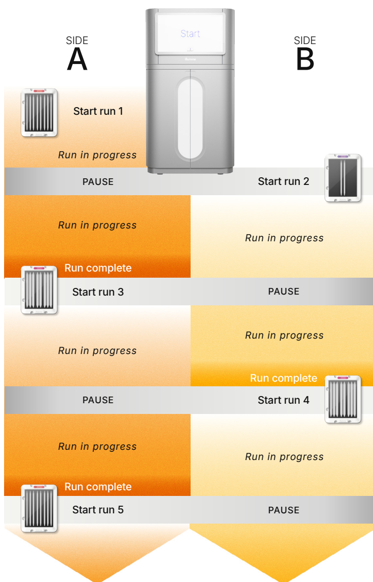
Figure 1: Staggered start on the NovaSeq X Plus supports continuous, near independent runs across all flow cell types and applications.
