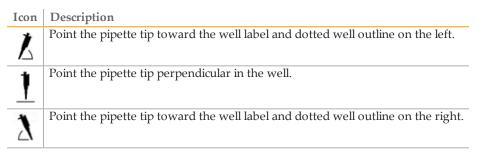
Increase the pipette angle if liquid is not dispensing from the pipette tips.
